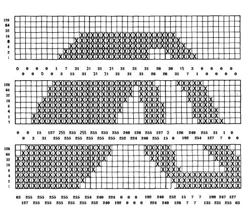
Following is the BASIC program that prints the design shown on the previous pages. Notice that the data numbers in lines **80-140** are the same numbers that you see in the last illustration. Also note that the WIDTH statement in line 10 is for IBM PC BASIC; the format may be different for your system.
